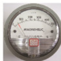
Differential Pressure Gauge Dwyer make Magnehelic gauges are used to measure the pressure drop HEPA filter 0-500Pa.
